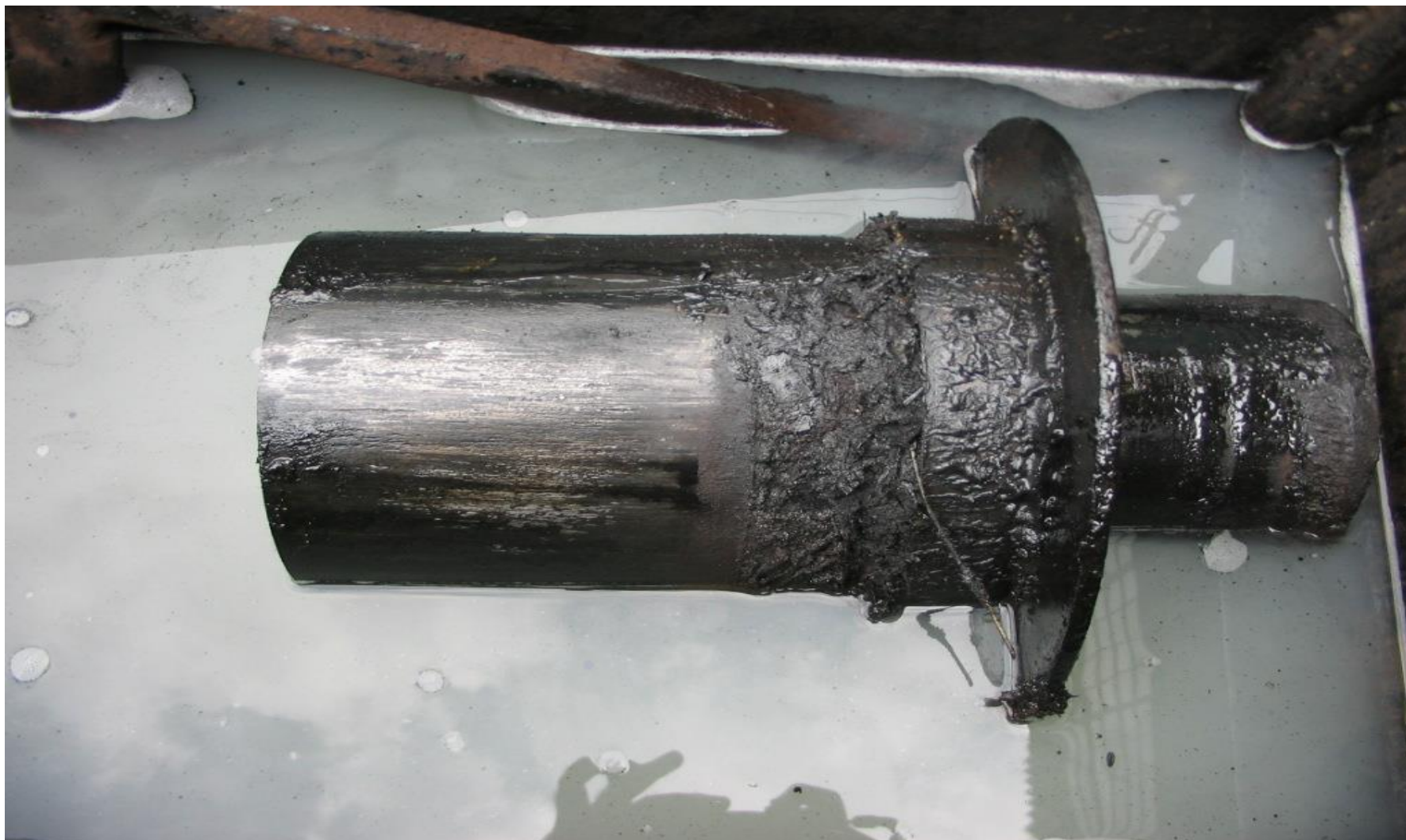
Dash Pot partially dipped in Ru ORA 7 for 30 minutes
