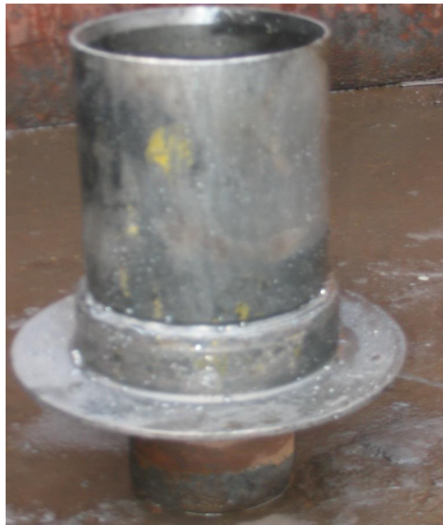
Portion of dash pot dipped in Ru ORA 7. Oil and sludge completely removed.
