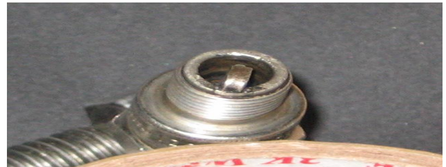
Removal of carbon from spark plug with Ru ORA 7
