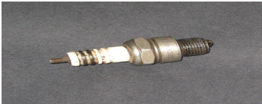
Removal of carbon from spark plug with Ru ORA 7
